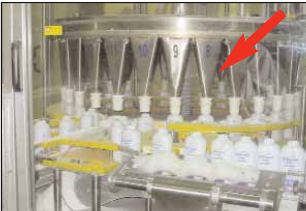
BVS-250 SILENT TURBINE VIBRATOR ON FILLING STATION increased fill rates and daily production by eliminating clogging of chutes.
