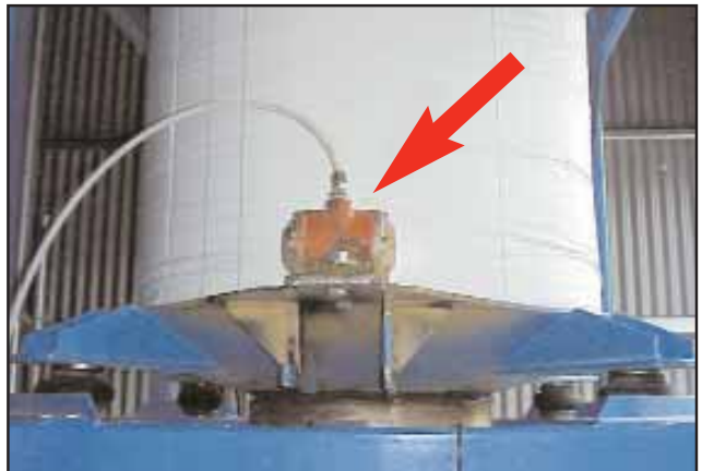
CCF-2000 SILENT TURBINE VIBRATOR ON FEEDER TUBE increased material flow and keeps it consistent. No more lost man hours to manual unclogging.
