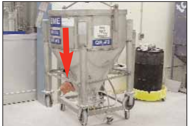
BVS-320 SILENT TURBINE VIBRATOR ON MOBILE BIN reduced batch contamination issues and clean up time. daily production increased significantly.
